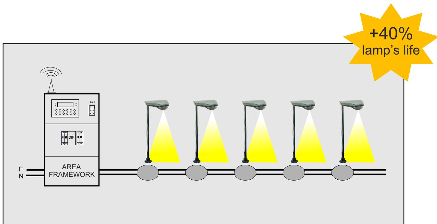
\* : Varibox system in combination with dimmable LED lamps.
